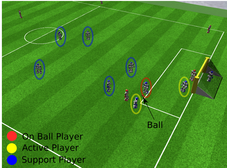
Figure 6.3: Defensive Positioning Resulting by Coordination Protocol, Example 1.
